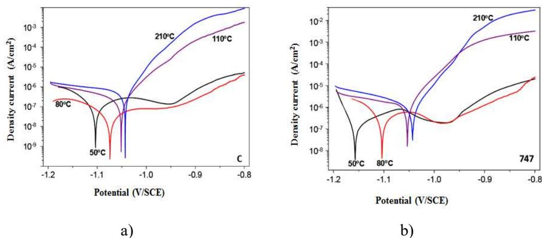
Figure 3. Polarization curves of conversion coatings produced in a - Cr (III) and b - conversion solution with various drying temperatures
