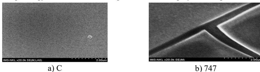
*Figure 2. Morphology of Cr(III) and Cr(VI) conversion coating surfaces*
